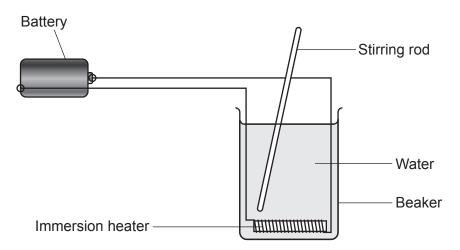
She uses an immersion heater to increase the temperature of the water.
